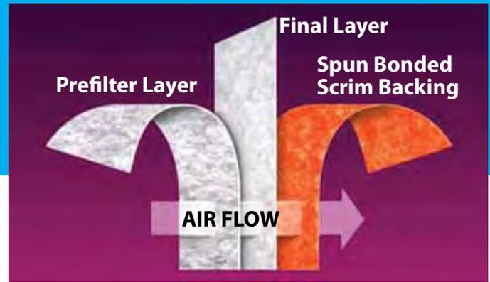
*Vari-Pak Model S dual layer synthetic media has a built in prefilter layer consisting of coarser fibers followed by a high efficiency final filter layer made of microfine fibers.*
